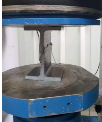
Figure ( 2): compressive test of (GFRP) model [28].
